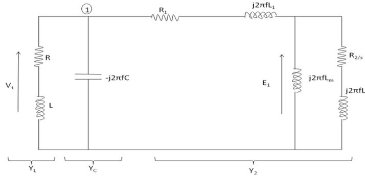
**Figure 1: Equivalent Circuit of Self-Excited Induction Generator**
